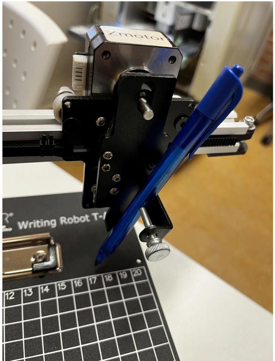
Once you're happy with the pen's position, tighten the clamp back up by turning the screw or knob clockwise (to the right). Make sure it's snug but not overly tight—you don't want to damage the pen or the clamp. Before starting your actual drawing, do a quick test run. You can do this by running a test plot or a simple line to see if the pen is drawing properly. If it looks good, you're all set! If not, adjust the height or the tightness of the clamp until you're satisfied.
