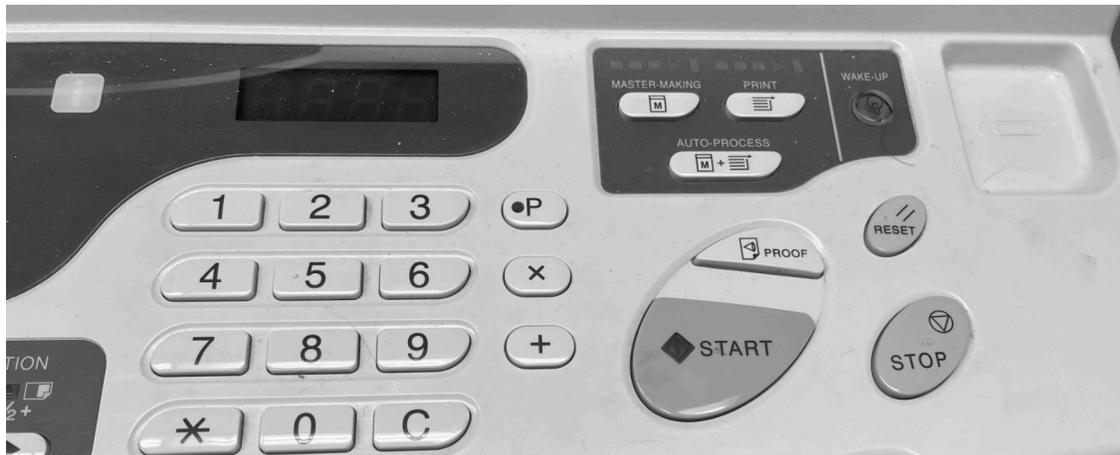
Image: Right panel of riso, with "Master-Making", "Stop", and "Reset" buttons, as well as number pad to input number of copies.
